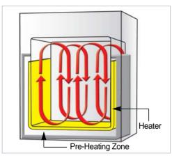
The Best Temp. Uniformity & Accuracy by High Performance Heating Mechanism (Gravity Convection-type)
